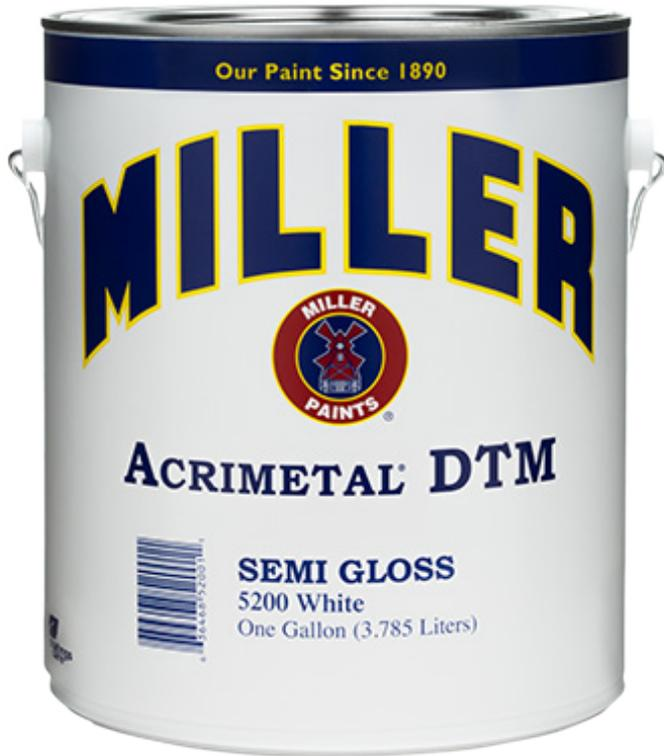
A premium, rust-inhibitive, interior/exterior acrylic coating. Acrimetal is formulated for direct application to bare metal and metal with tight rust. Acrimetal is extremely durable, has excellent adhesion to metal and galvanized surfaces and contains rust inhibitive pigments for added protection. It is a versatile replacement for conventional solvent-borne industrial primer/finish systems.
